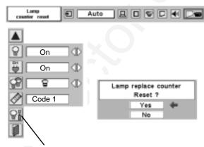
Move the pointer to Lamp counter reset and then press SELECT button. The message "Lamp replace counter reset?" is displayed.
